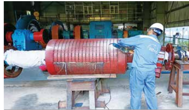
GENERATOR Renew Rotor Windings Power: up to 15 MVA - Voltage: up to 6600 V
