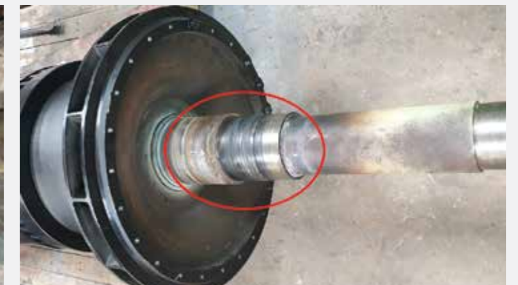
Power: 500 kW Voltage: 6600 V Restore Shaft and flame path
