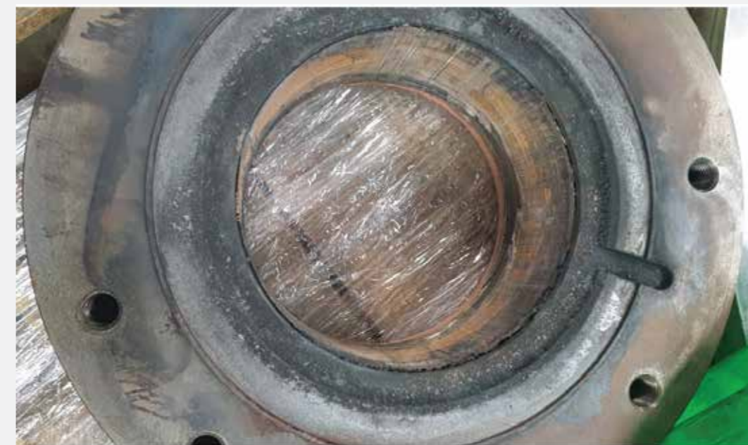
Power: 500 kW Voltage: 6600 V Visual Inspection - Detail Inspection - Restore shaft - Restore bearing cap - Balance
