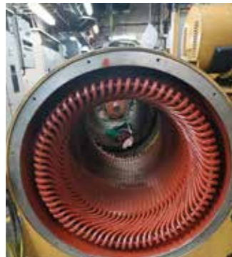
STATOR Checking - Cleaning - Drying - Varnish Insulation
